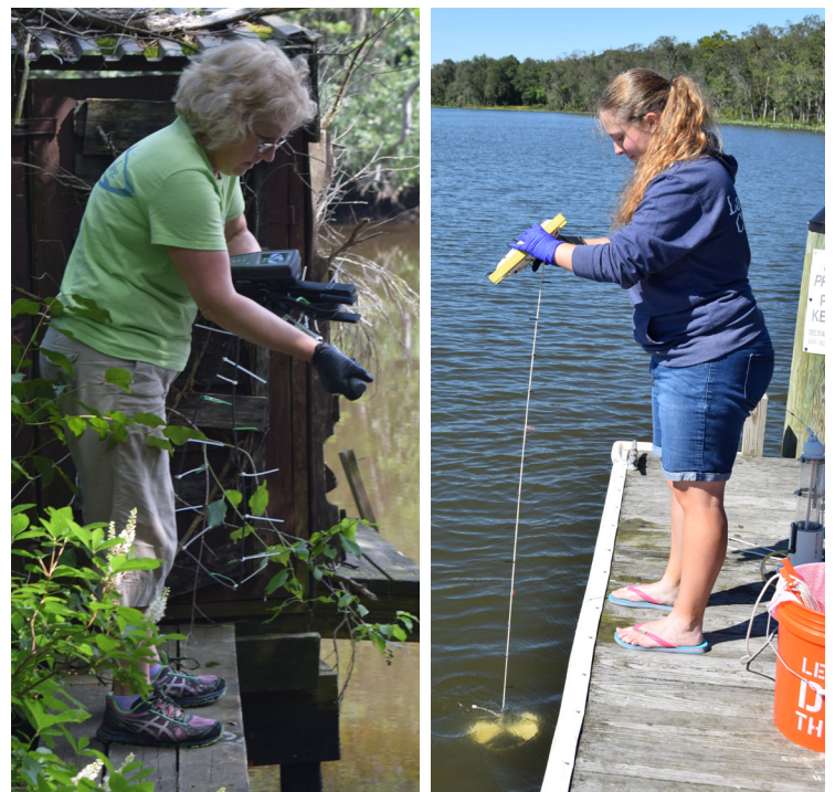
Figures 11-12 (above): (l) Creekwatcher Nan Zamorski measures dissolved oxygen at an upper Nanticoke site, while (r) Creekwatcher Helen Wilson uses a Secchi disk to obtain water clarity and total water depth measurements.
